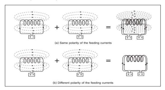
The concept used in this experiment is an fundamental physics; it is about the magnetic field **B** generated by a direct current flowing in a solenoid as show in the diagram and according to the formula,
